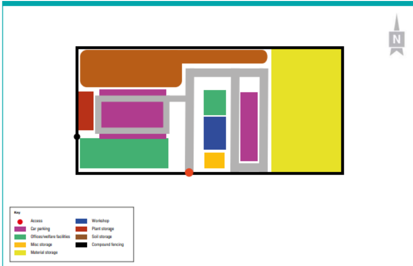
Plate 1.18 Utility Logistics Hub indicative layout
